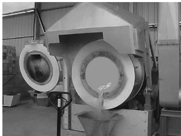
Fig. 8. Tap out of raw lead from tilting rotary reduction furnace.
