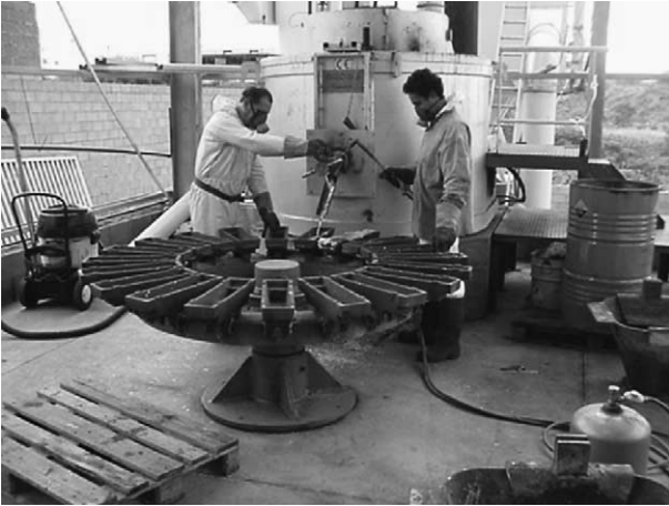
Fig. 9. Ingot casting from refining kettle.
